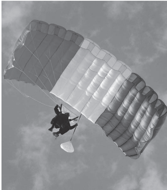
FIGURE 1.13 Since its development during World War II, nylon fabric remains the most popular material of choice for parachute designs. (Courtesy of Stringer/Agence France Presse/Getty Images.)
